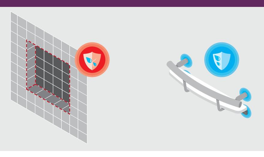
Built-in Niches have many tiled seams that must be sealed to prevent water penetration. The seams can be long in length and numerous, with the responsibility on the contractor to ensure the seal is 100% water tight.
